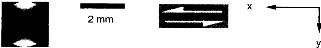
Fig. 2. First and last image of stack of IT-HS experiment on norcamphor (IT-HS = intermediate temperature, high strain rate). Images were taken with a 'Wild Photoautomat' camera. Traces for slicing at y = 40, 110, 130, 150 and 200 are indicated. Grey values correspond to crossed polarizer conditions (yellow = bright, magenta = dark, blue = intermediate grey). For details of experimental conditions and polarizer orientation, consult Herwegh et al. (in press). Inset: stereographic representation of the grey values.
